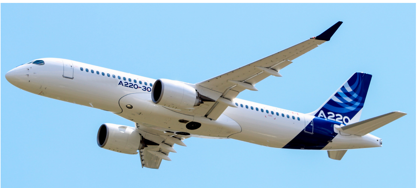
The Airbus A220 uses Pratt & Whitney geared turbofan engines that are some of the quietest and most fuel-efficient engines currently in production.
