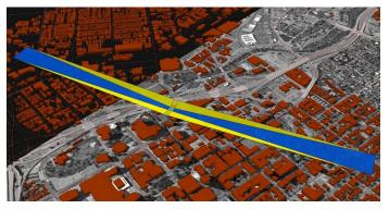
Penetrations could be mitigated by realigning the approach/departure paths, or removal, lowering, or lighting of the penetrating object.
